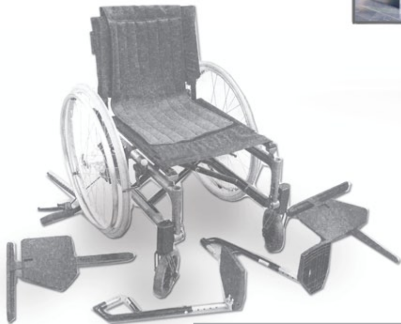
Traditional wheelchair in steel - Loose parts often missing when needed
